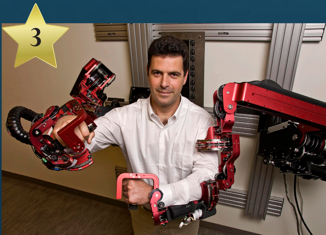
3 University of California at Santa Cruz, Santa Cruz, CA, USA. Powered upper-limb exoskeleton. This presents a new model, using a full body immersive surgeon's console for telesurgical user interfaces.
