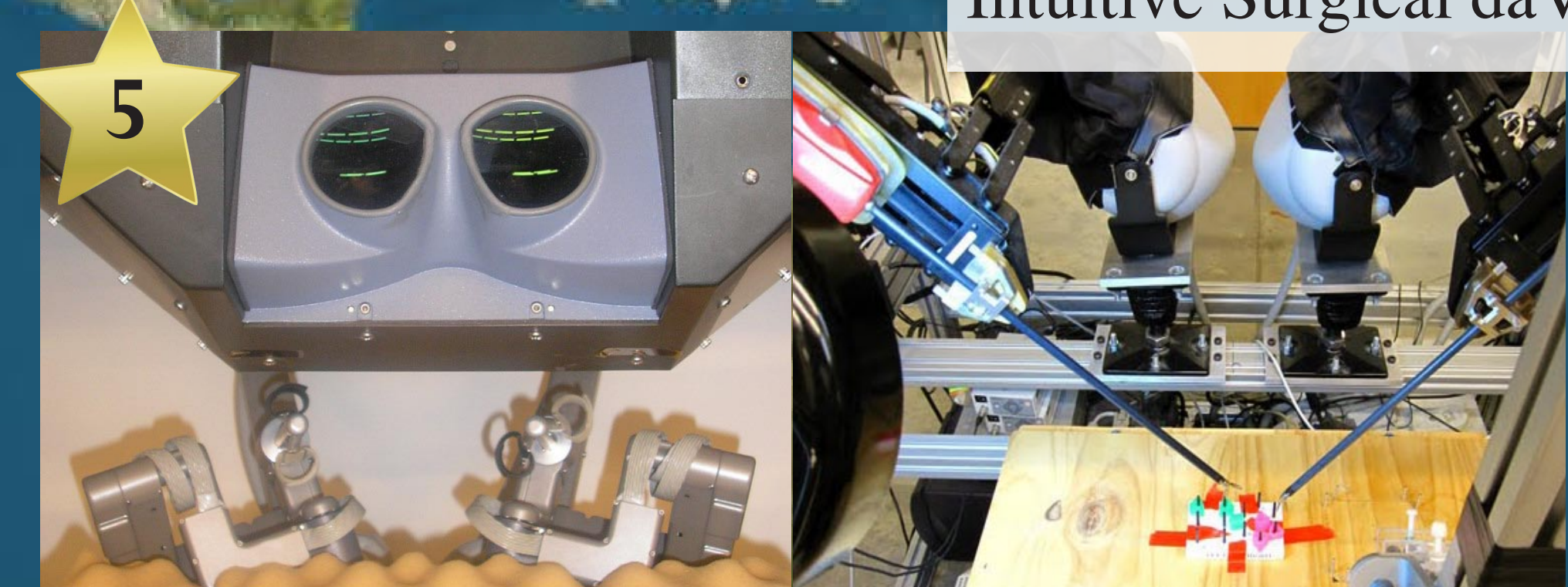
5 Johns Hopkins University, Baltimore, MD, USA. JHU Custom daVinci master and slave system. This is a research version of the state-of-the-art daVinci robot by Intuitive Surgical daVinci.
